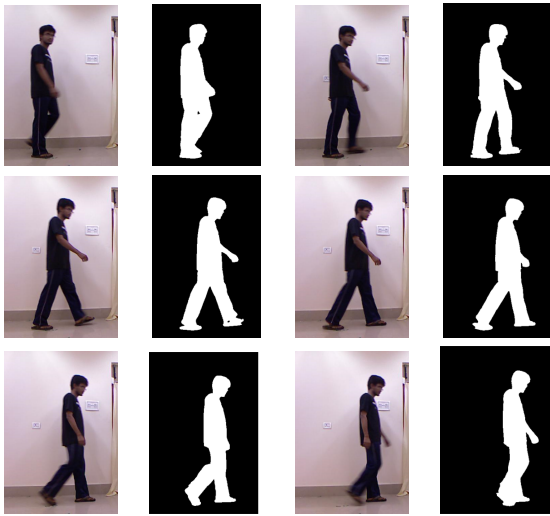
Figure 4: 6 Frames depicting the half-gait-cycle of the subject alternating with the silhouettes from respective frames.
